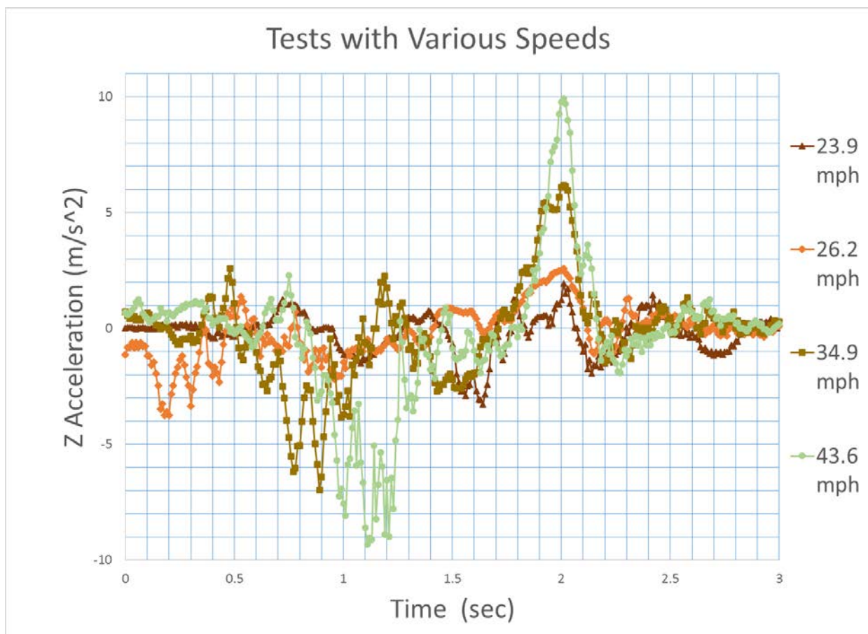
FIGURE 7. Accelerations Measured at Various Speeds.
